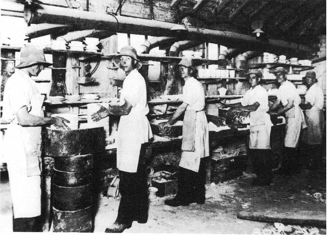
65 Placing the 'green' ware into saggars, using some individual bedders, c. 1930
