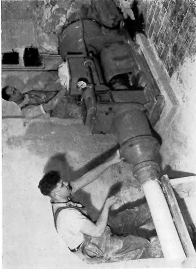
The "Pug Mill" which kneads the clay to the requisite consistency and removes any imprisoned air bubbles.
