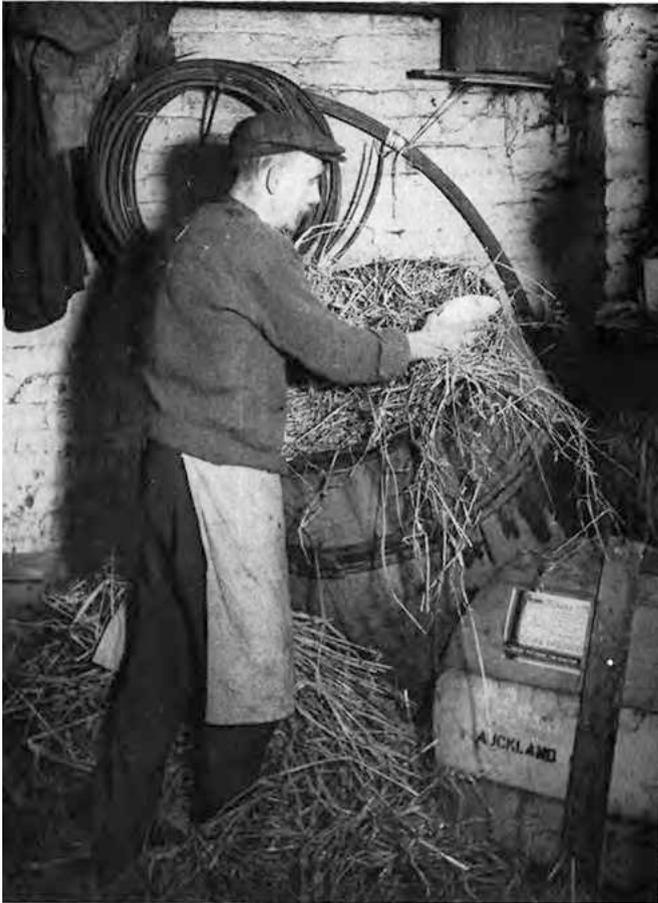
Packing for Export. As no china can withstand, unprotected, the rough treatment which it receives in transit; it must be very carefully packed. Shelley packers are experts in the use of straw and wood wool as shock absorbers
