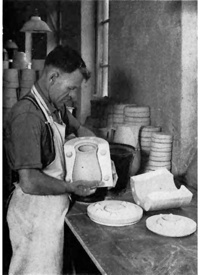
Removing the cast article from the mould after drying
