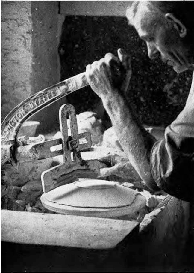
The Platemaker. Plates and saucers are made on a jigger upside down on a mould which shapes the upper surface or face of the article. A specially shaped tool which is pressed down by the operative, squeezes out the clay to the desired thickness, and shapes the back or underside
